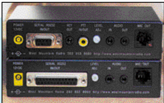
Rear view of the RIGblaster (bottom) and RIGblaster Plus (top) show additional jacks added on the Plus version. See text for details.
